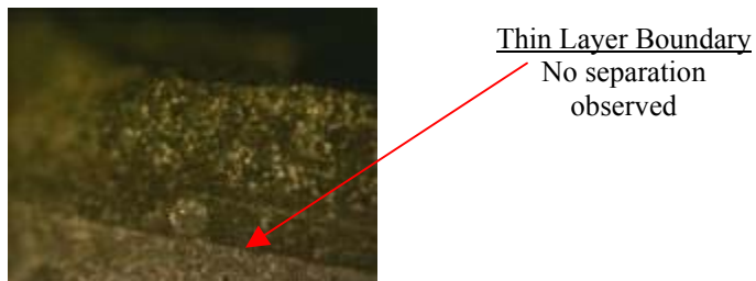
Figure 14: Cross Section of 1.30:1 Glow Powder, 1.9:1 Water after Three Point Bend Test
