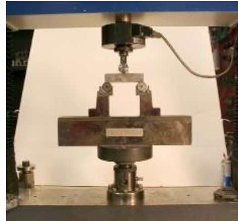
b. Photo of Three Point Bend Testing Setup (Photo Courtesy of Mark Seniw)
