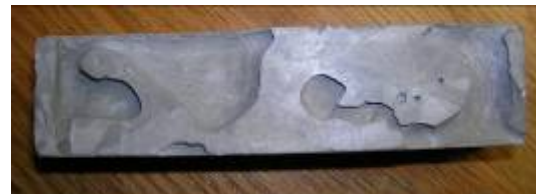
Figure 4: Samples with Irregular Surfaces Caused by Air Bubbles
