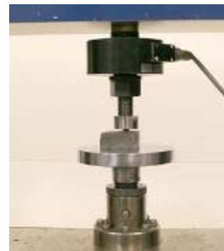
b. Photo of Compression Testing Setup (Photo Courtesy of Mark Seniw)
