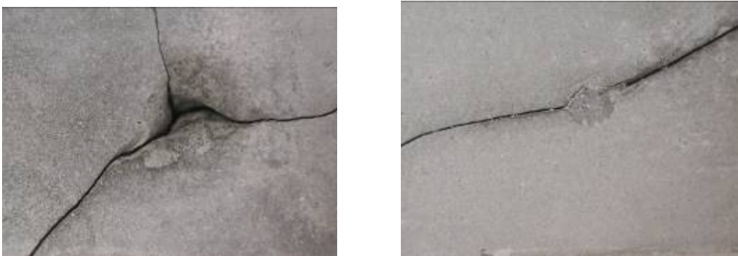
Figure 16: Representative Compression Test Results – Poor and Good Adhesion 1.30:1 Glow Powder Ratio, 1.7:1 Water Ratio– example of poor adhesion (left); 2.5:1 Glow Powder Ratio, 2.1:1 Water Ratio – example of good adhesion (right)
